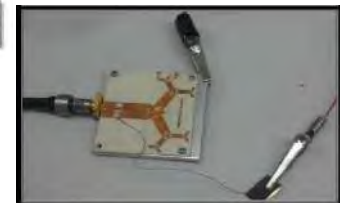
Fig. 3: Prototype of Reconfigurable Fractal Tree Antenna
