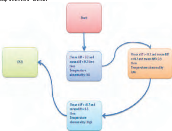
Fig.6. Algorithm of Temperature Data Processing
