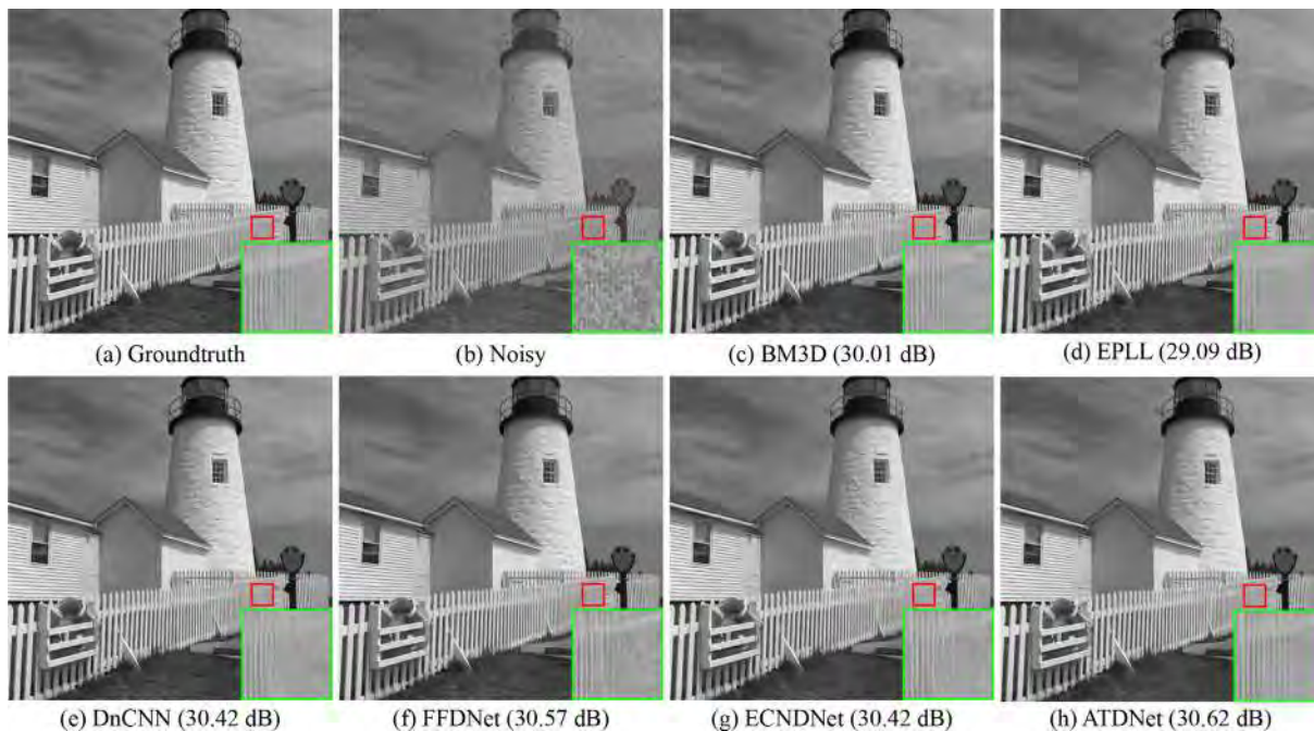
Fig. 12. Denoising results of a gray image from Kodak24 dataset with noise level 25 dB.
