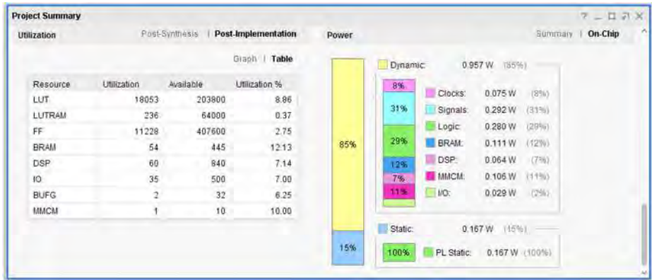
Fig. 18 Resource utilization and power estimation from post-implementation
